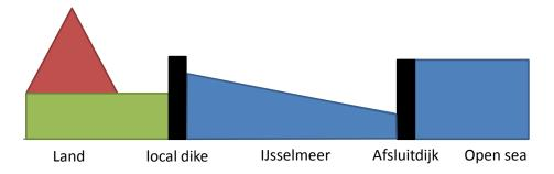
Optimal construction: inner dike at norm, outer dike can be far weaker.
